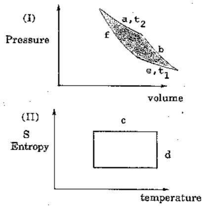
Figure II represents the Carnot cycle in a S-T diagram. Curves a and e are isotherms for temperature  $t_2$  and  $t_1$ , respectively. For curves a, b, c and d which curves represent an adiabatic process. (A) a, b, (B) a, c (C) b, c (D) b, d (E) c, d
