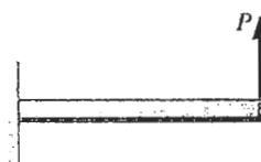
$$v = \frac{Px^2}{6EI}(3L - x) \quad v' = \frac{Px}{2EI}(2L - x)$$
