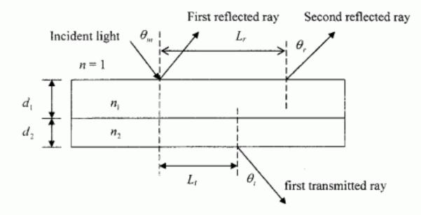
9. (5%) A dielectric slab waveguide in vacuum has a refractive index of 1.5, as shown below. What is the maximum angle of an incident light within which the light can be guided in the waveguide?
