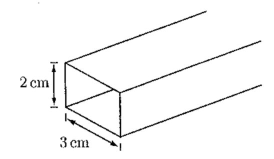
(a) What is the fundamental mode of this waveguide?
