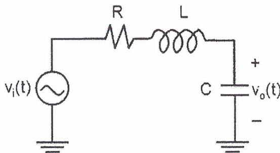
You are required to calculate the input frequency  $\omega_o$  that will cause the output  $v_o(t)$  to have an exact  $90^\circ$  phase delay with respect to the input  $v_i(t)$ , as the output reaches its steady state (namely, the particular solution of the differential equation).
