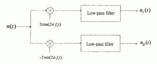
where the low-pass filters are ideal with a bandwidth equal to one-half that of the narrowband noise n(t).
