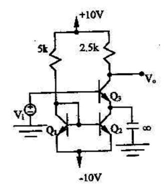
An amplifier can be modeled by the equivalent circuit as shown. Find the input impedance Z<sub>k</sub> and the pole of V/V<sub>i</sub>.
