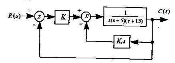
please design the inner-loop feedback compensation (i.e.,  $K_i$ ) to yield a damping ratio of 0.8 for the inner-loop (in this case there are three complex poles at  $0,-10 \pm j7.5$ ) and then design outer-loop feedback compensation (i.e., K) to yield a damping ratio of 0.6 for the closed-loop system (in this case there are three poles at  $-10.93,-4.535 \pm j6.046$ ). (15%)
