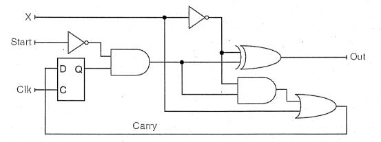
b. (4%) What is the shortest operation time for the circuit if you designed for a 64-bit operation? Assume the delay time for D Flip-Flops, NOT, AND, OR, and XOR gates are 180ps, 4ps, 120ps, 100ps, 140ps, respectively. You may ignore the flip-flop setup time.
