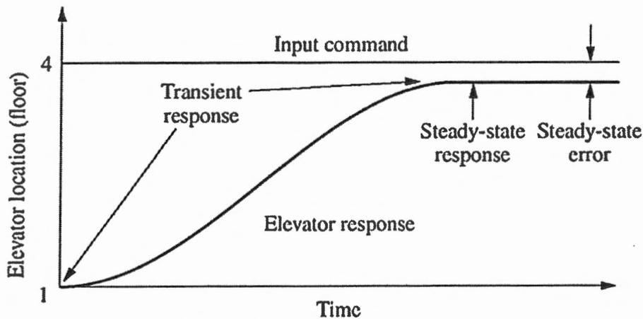
FIGURE 1.2 Elevator response
