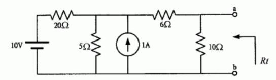
33. Find current I in the following circuit. I= (a) 8A (b) 9A (c) 10A (d) 11A (e) 12A.
