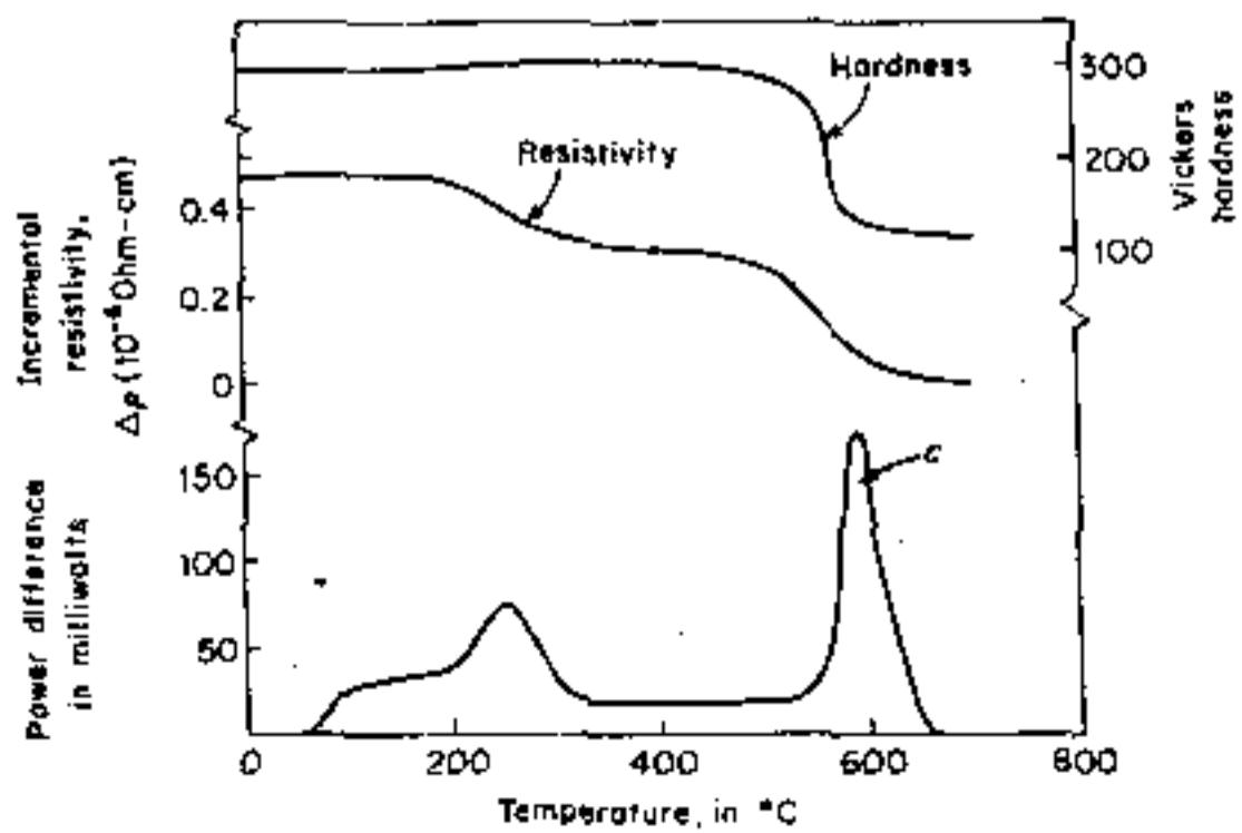
**图二.** Anisothermal-anneal curve for cold-worked nickel. At the top of the figure curves are also drawn to show the effect of annealing temperature on the hardness and incremental resistivity of the metal. (From the work of Clarebrough, H. M., Hargreaves, M. E., and West, G. W., *Proc. Roy. Soc., London*, 232A 252 [1955].)
