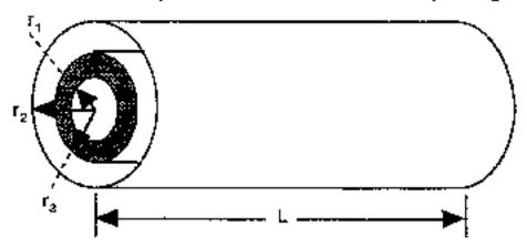
3. (10 points) A long coaxial cable (shown in cross section) has a uniform current I flowing in the center conductor into the paper, and the same current I flowing in the outer cylinder out of paper.
