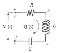
Remark: R: resistance, L: inductance, C: capacitance, Q(t): charges, V(t): voltage drop
