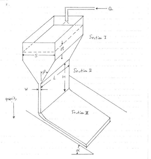
The same liquid in the above problem now flows into a tank with a converging section as shown in the figure, the angle  $\beta$  is less than 15°. All the dimensions are shown in the figure. Assuming steady, one-dimensional fully developed flow exists in sections II and III, what is the maximum velocity in Section III? List your assumptions. Note that L>>W, H>>W, S>>W, you may neglect end effects. (10%)
