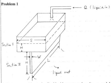
A dilute aqueous Newtonian liquid with constant viscosity  $\mu$  and density  $\rho$  flows into an open rectangular tank with two sections. The dimensions of both sections I and II are shown in the figure. Assuming L>>W, H>>W, S>>W, steady one-dimensional fully developed flow exists in Section II, you may also neglect edge and entrance effects. What should be the inlet volumetric flow rate Q to maintain the liquid level at a constant level M in section I? List your assumptions. (10%)
