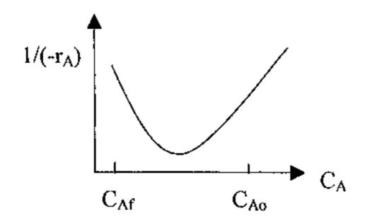
For a reaction with reaction rate curve as shown ( $C_A$  is the concentration of reactant,  $-r_A$  is the reaction rate), the volumetric flow rate ( $v_o$ ), the initial and final reactant concentrations,  $C_{Ao}$  and  $C_{Af}$ , are known.
