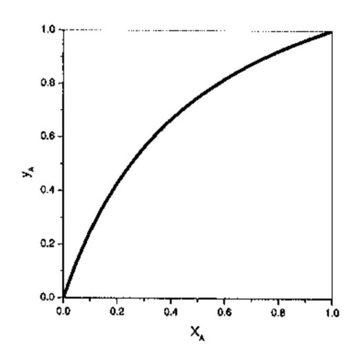
The above is a y-x diagram of a binary liquid mixture containing A. What is the minimum number of stage when a mixture of 50 mol% A is separated into a stream containing 90 mol% A, and another stream containing 10 mol% A.
