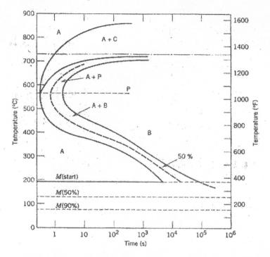
In the following case assume that the specimen begins at 1690°F and that is has been held at this temperature long enough to have achieved a complete and homogeneous austenitic structure.
