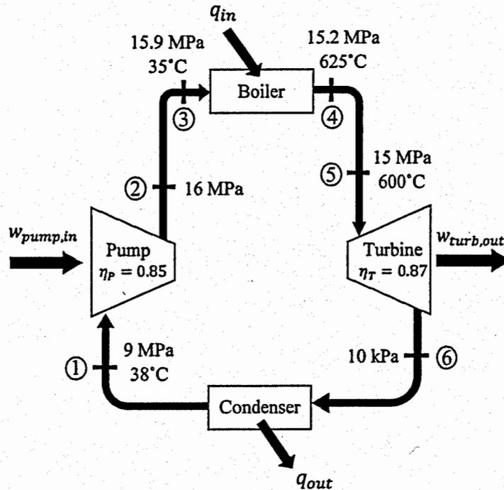
Q4-1. Sketch an ideal temperature-entropy diagram, where a loop of the working fluid circulates through the four components. Indicate the constant-pressure processes and three zones: compressed liquid, liquid-vapor mixture and superheated vapor.
