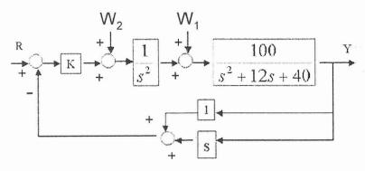
(c) Based on the Ziegler-Nichols Tuning method (Table 4.2 on the next page), design a PID controller  $G_c(s)$  instead of proportional controller K. (10%)
