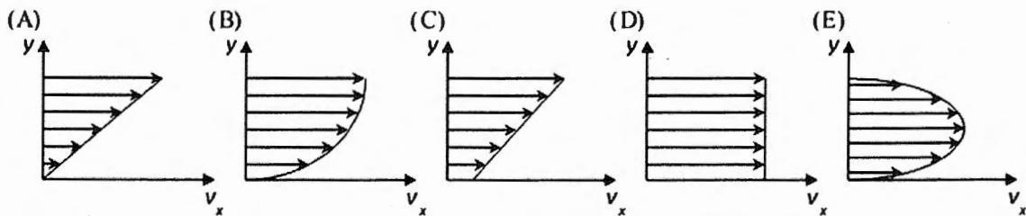
4. Following the above question, consider the flow of water ( $\mu = 1 \text{ cp}$ ) with upper plate of surface area equal to  $0.5 \text{ m}^2$  and the velocity of the upper plate ( $U$ ) equal to  $2 \text{ m/s}$ . If the separation distance between the two plates ( $b$ ) is equal to  $2 \text{ mm}$ , calculate the rate of viscous dissipation ( $\text{J/s}$ ).
